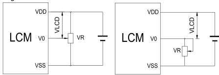
V<sub>DD~</sub>V₀: LCD Driving voltage
